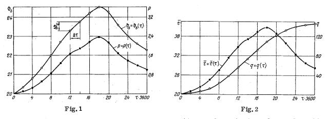
Fig. 1. Vessel temperature over housing temperature  $\vartheta_{s}(\tau)$ , °C and specific thermal power loss  $p(\tau)$ , W/kg as functions of time  $\tau$ .
